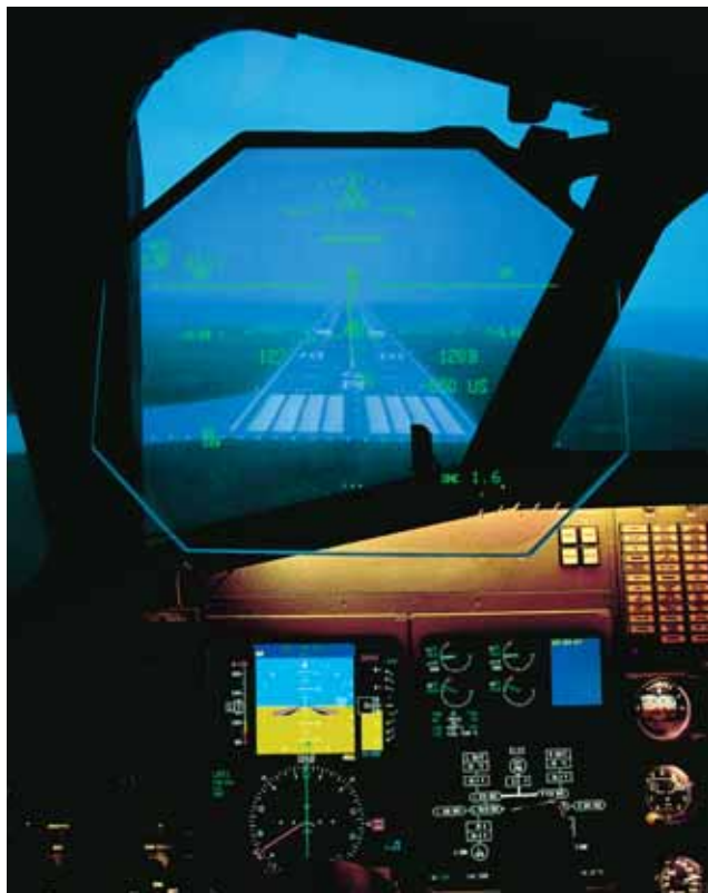
Figure 6-13. Head-up Guidance System.
