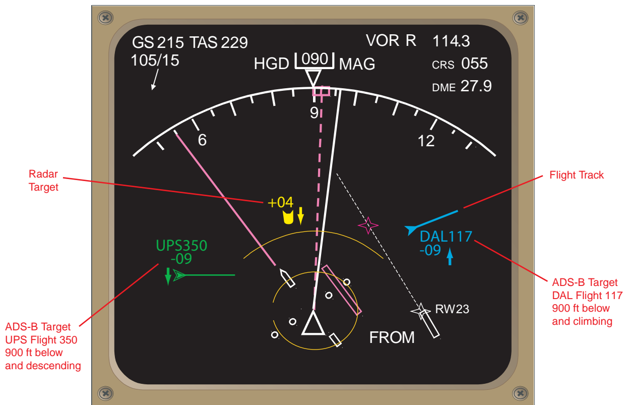
Figure 6-7. Cockpit Display of Traffic Information. This display shows both ADS-B and other aircraft radar targets.
