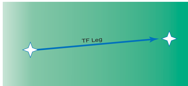
Figure A-7. Path/Terminator. A Path/Terminator value of a TF leg indicates a great circle track directly from one fix to the next.
