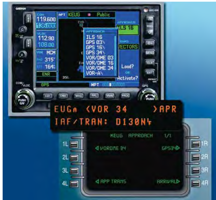
Figure A-2. Naming Conventions of Three Different Systems for the VOR 34 Approach.
