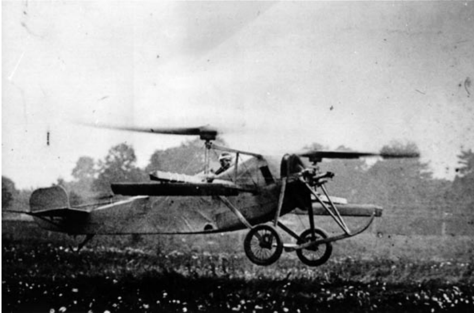
Figure 1.5 This Berliner helicopter with side-by-side rotors made short flights at College Park airport in Maryland in 1922. (Courtesy of College Park Airport Museum.)
