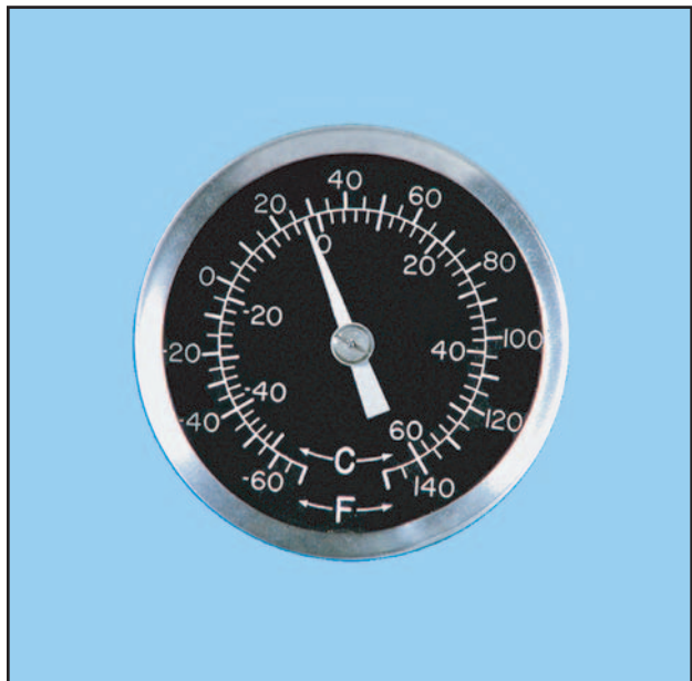
Figure 6-24. Outside air temperature gauge.
