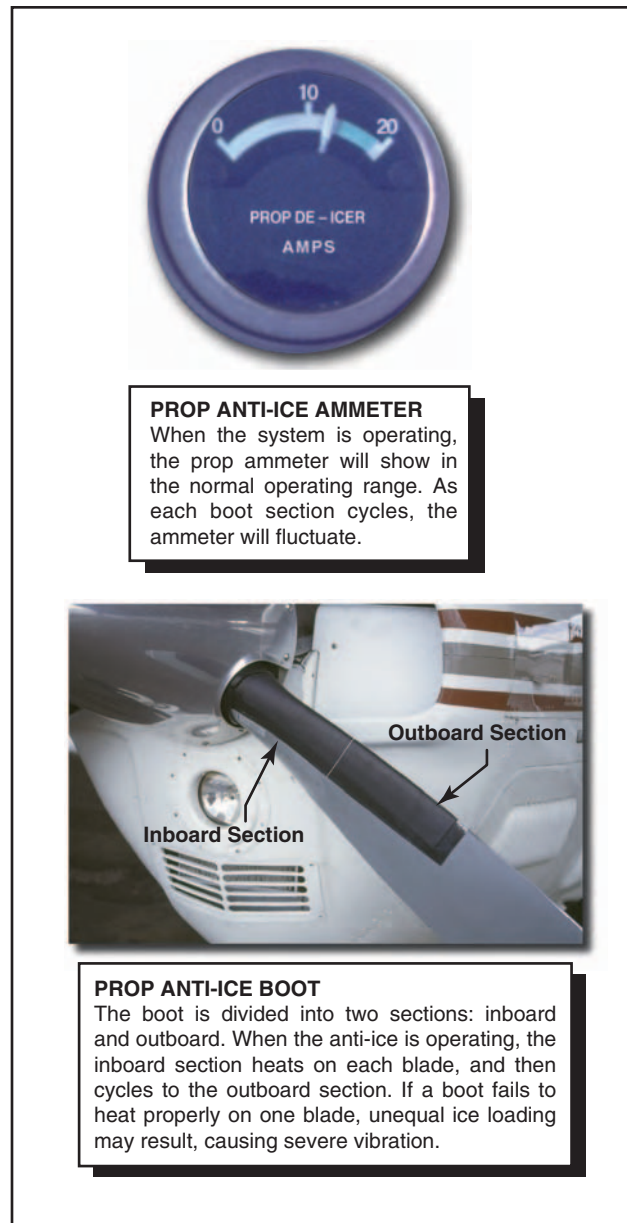
Figure 5-35. Prop ammeter and anti-ice boots.
